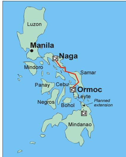
National Power Corporation has constructed a 440 MW, 350 kV monopolar HVDC link to transfer power from the geothermal power plant on the island of Leyte, to the southern part of the main island of Luzon to feed the existing AC grid in the Manila region.
