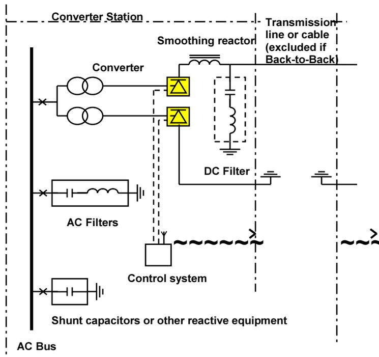
**The converter station:** The converter stations at each end are replicas of each other and therefore consists of all the needed equipment for going from AC to DC or vice versa. The main component of a converter station are:
