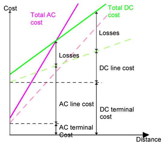
The breakeven distance depends on several factors, as transmission medium (cable or OH line), different local aspects (permits, cost of local labour etc.). When comparing high voltage AC with HVDC transmission, it is important to compare a bipolar HVDC transmission to a double-circuit high voltage AC transmission, especially when availability and reliability is considered.
