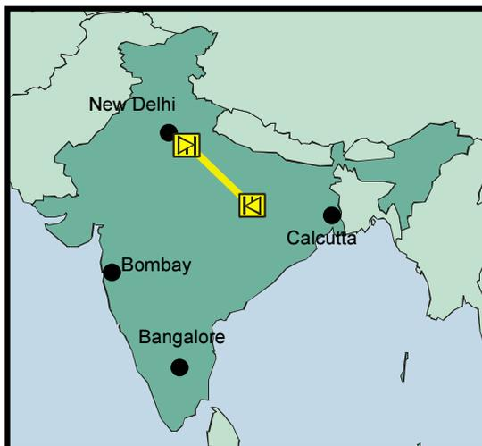
National Thermal Power Corporation Limited built a 3000 MW coal-based thermal power station in the Sonbhadra District of Uttar Pradesh State. Part of the power from the Rihand complex is carried by the Rihand-Delhi HVDC bipolar transmission link, which has a rated capacity of 1500 MW at  $\pm 500$  kV DC. Some of the power is transmitted via the existing parallel 400 kV AC lines.
